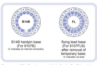
Our range of B14B sockets, available for the B14B hardpin base, includes versions with or without a mounting flange, and versions with contacts for mounting directly onto printed circuit boards.
